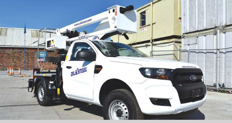
A highly stable platform for working up to a maximum height of 13.8m, with a maximum working outreach of 7m
