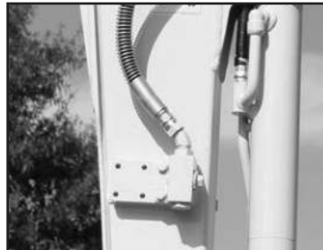
Auxiliary Hydraulic Lines
