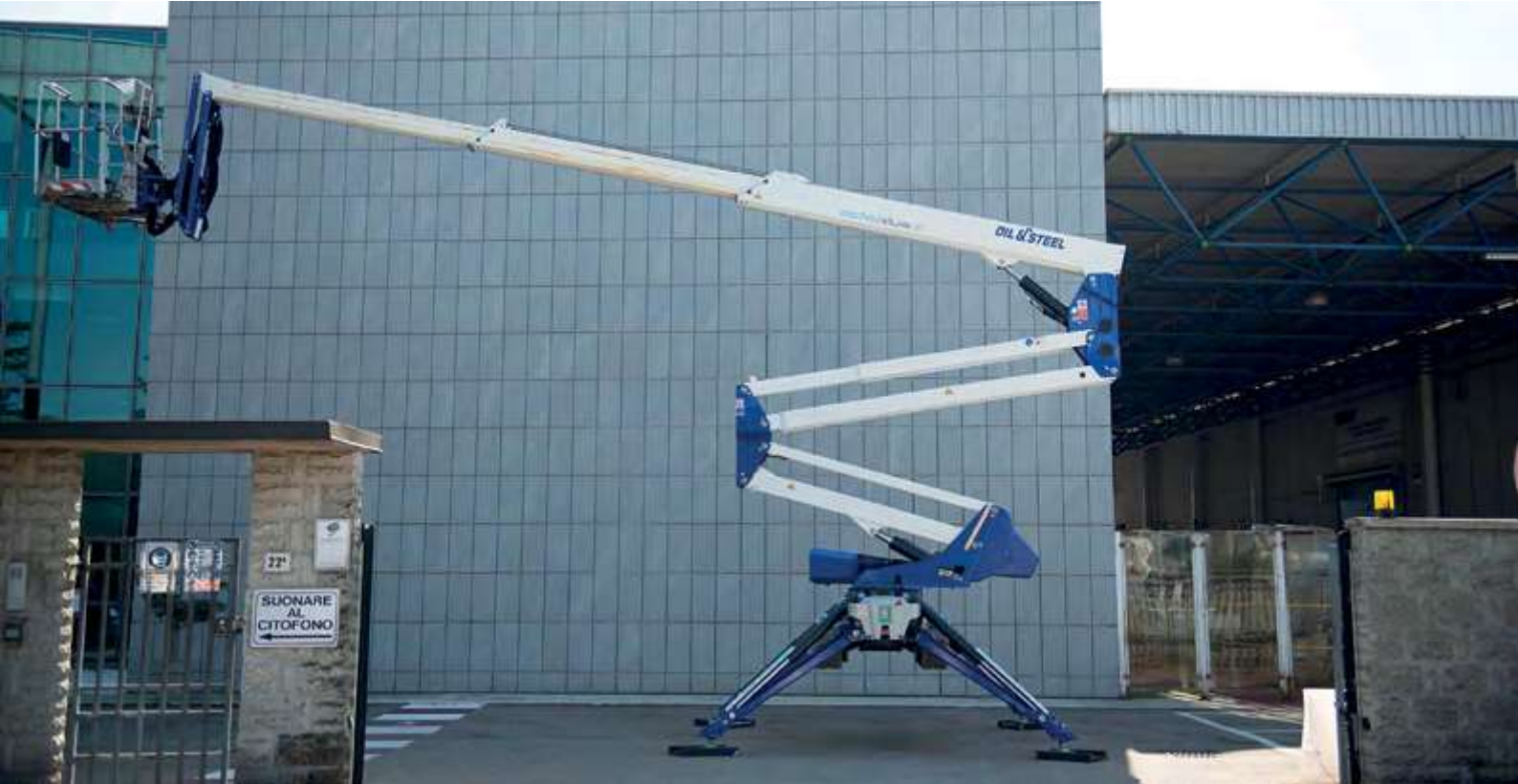
Exceptional ground clearance and a maximum working height of 21m – the Octoplus 21 delivers industry-leading performance
